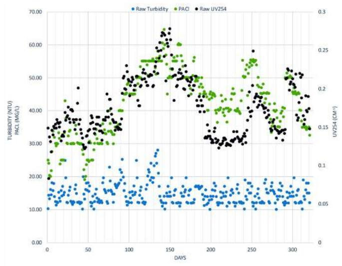
Figure 1: Real-time raw water organics in comparison to turbidity displays need for both measurements to effectively treat water.
