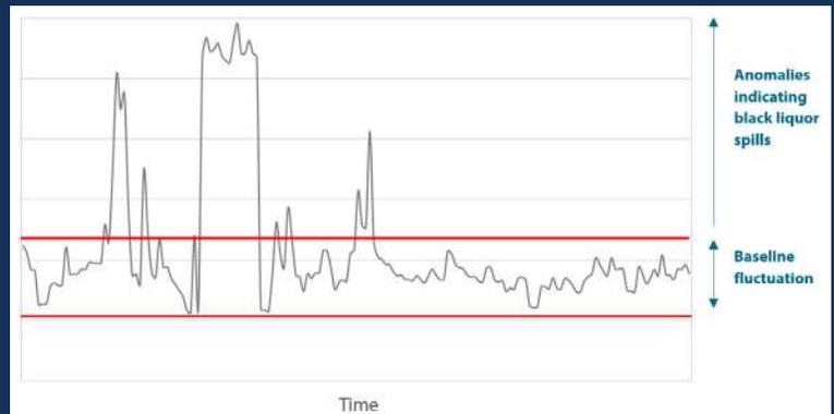
Fig. 3: Real-time data over time showing how the normal baseline fluctuation in the wastewater composition is distinguished from an overnight black liquor spill event.
