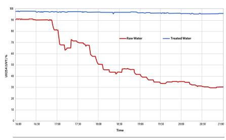
Figure 3: Data from Real Tech's dual feed UV254 analyzer. UV transmittance (UVT%) readings from raw water (red) compared to treated water (blue) visualize treatment efficiency for operators.
