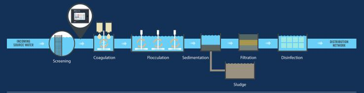
Figure 2: The typical installation point for raw water quality monitoring at a conventional drinking water treatment plant. Real Tech's dual feed upgrade allows for monitoring at two locations within the plant with a single UV254 analyzer.
