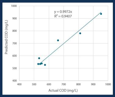
FIG. 2: A regression analysis showing the predicted COD results from the Real Tech system plotted against the laboratory COD results.
