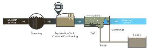
Fig. 1: A process diagram of the plant's wastewater treatment train showing where Real Tech's monitoring system is located.
