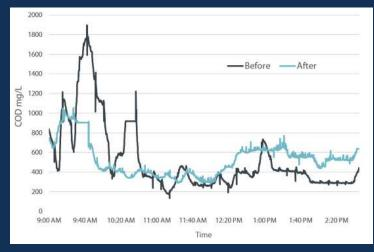
Fig. 3: Daily real-time data comparing COD before (black) and after (blue) cleaning cycle process improvements.
