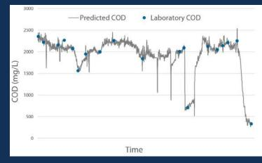
Fig. 2: Displays the real-time predicted COD data from the sensor in grey and laboratory COD grab sample data taken over the same period in blue.
