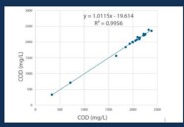
FIG. 3: Displays a comparison of 19 laboratory sample results for COD and the corresponding predicted COD results from the sensor. The R2 value of 0.9956 suggests a high accuracy in the predicted real-time data.
