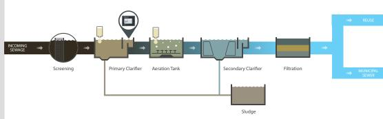
FIG. 1: A process diagram of the plant's wastewater treatment train showing where Real Tech's monitoring system was sampling from.
